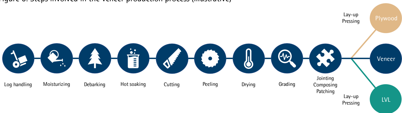
Figure 6: Steps involved in the veneer production process (illustrative)
